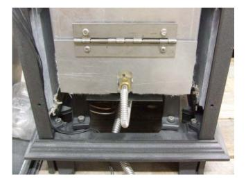
12. From the front of the stove, pull the control valve forward far enough to access the pilot and thermocouple connections at the rear of the control valve.
