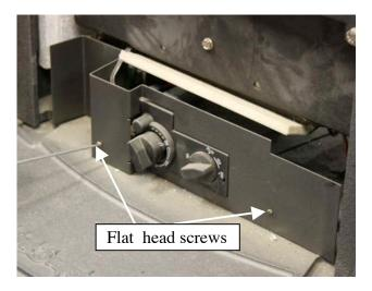
6. Use a 5/32" allen wrench to remove all six of the screws fastening the rear panel to the back of the stove. One of the six is the screw that also holds the switch box in place and must be accessed through the upper hole in the switch box.
